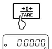
Unload the balance. Press the **TARE** key.
