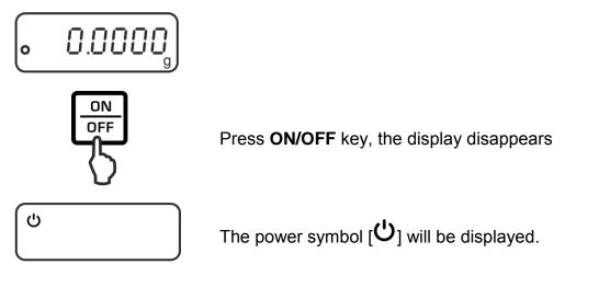
In stand-by mode the balance is ready for operation immediately after switching-on without warm-up time.
